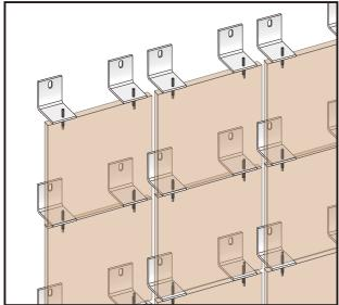
The fit pin is fixed by press machine in workshop. This ensure all the S.S. pins are vertical, in a good shape and could be held tightly in the bracket.
