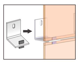
The fit plate is fixed by press machine in workshop. This ensure all the S.S. plate are vertical, in a good shape and could be held tightly in the bracket.
