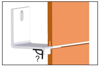
If the fold angle is not 90 degree, a gap may formed between two stone panels. This may affect the appearance of the whole stone facade.
