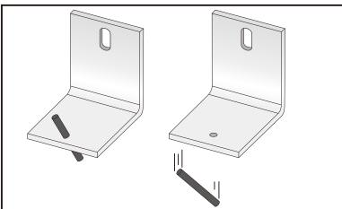
Pin may not be vertically fixed in the bracket or may be lost during the installation process.
